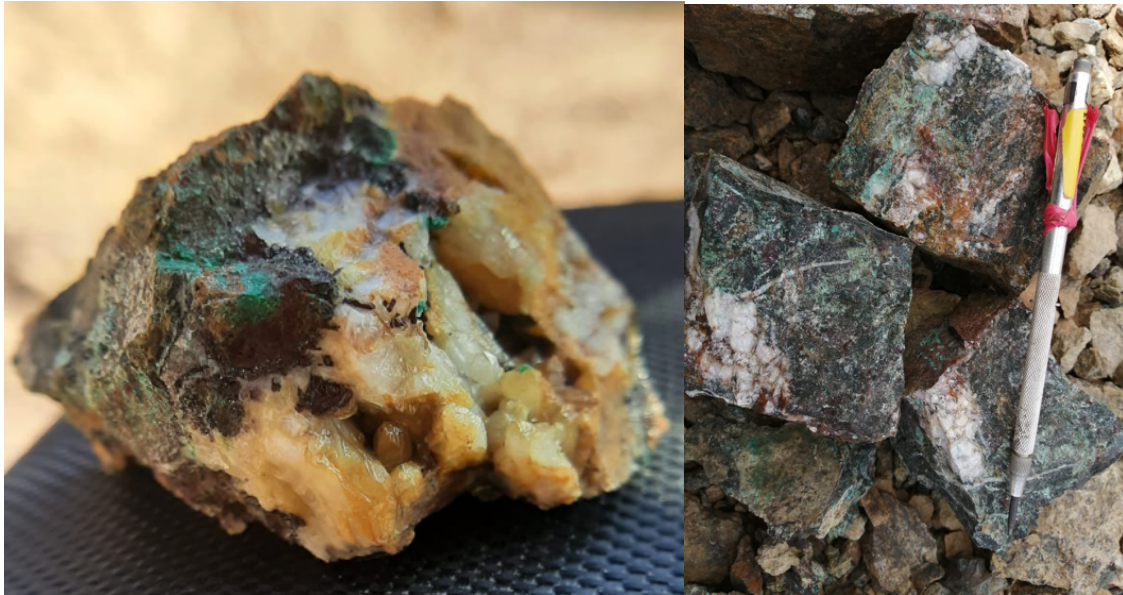
Photos 1 & 2. Hand sample in the surface vein, quartz, malachite and chocolate formation
