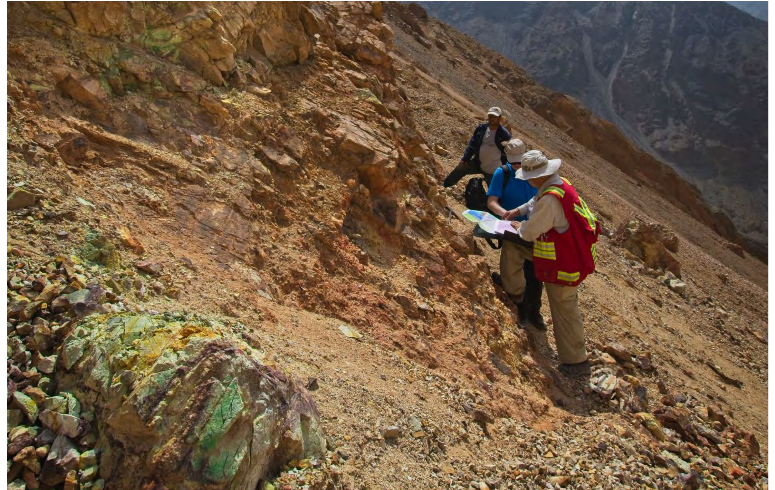
Green copper oxide mineralization in outcrops on the east side of Target 1.
