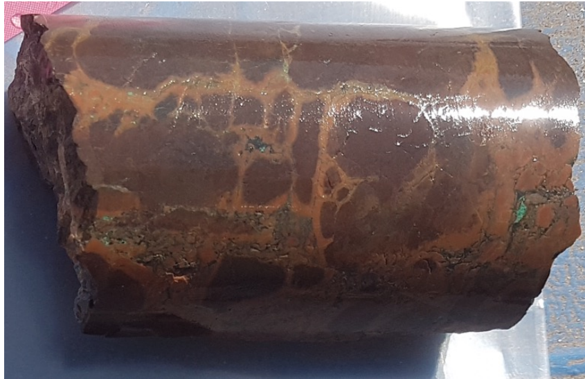
Photo 2. Petrographic cut sample from hole DCH-001 at depth from 282.95 m to 283.05, grade up to 1.06% Total copper and 1.02% Soluble copper in the core interval 282 m to 283.5 m.
