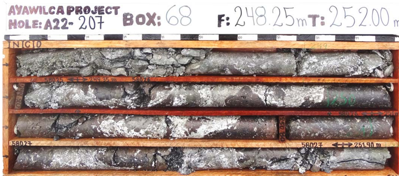
Figure 4. Drill core of breccia-hosted zinc sulphides (brown colour) in drill hole A22-207 with interstitial carbonates and clays (white colour).
