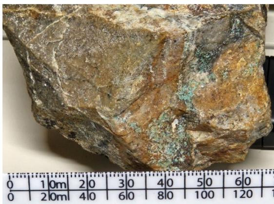
*Figure 5: Hornfels with fine quartz veinlets, weak disseminated biotite, Fe oxides (goethite) in fractures, green Cu oxides (malachite) and black Cu oxides in fractures and disseminated (262120E, 8060419N)*
