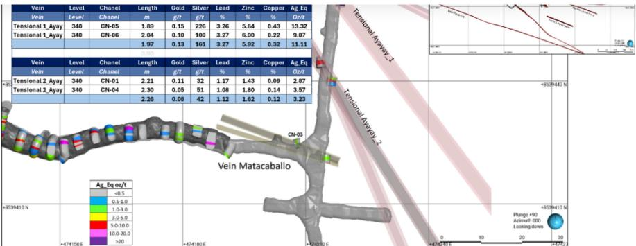
Figure 1: Detail plan at 340 level showing sections of the Ayayay and Matacaballo vein systems
